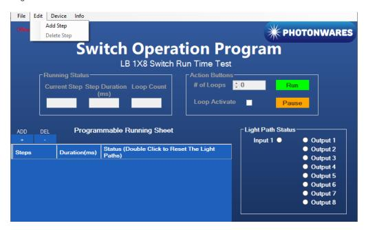
**Edit step**: There are two things that you can modify for one step. One is the light path, and the other is the duration for each step. Double click the cell that you want to modify, and the program will allow you to modify the setting.
